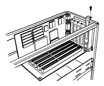
2. Slide out the slot cover and set it aside. (Store it in a safe place in case you remove the option card later.)
